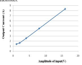
Fig 13. Amplitude of Input Vs output current
