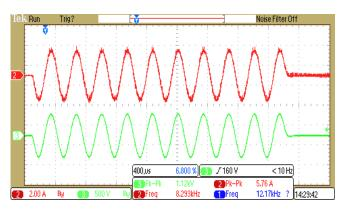
Fig.9. Output voltage and current waveform of power amplifier without feedback for 225  $\!\Omega$  load.
