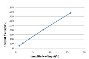
Fig 14. Amplitude of Input Vs Output voltage
