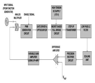
Fig.7. Power amplifier with analog feedback controller
