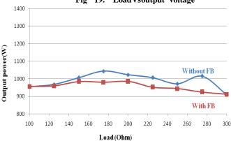
Fig 20. Load Vs output power
