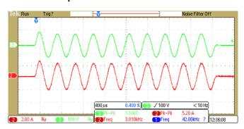
Fig.10. Output voltage and current waveform of power amplifier with feedback for  $225\Omega$  load
