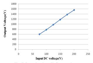
Fig 18. Input dc voltage Vs Output voltage
