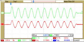
Fig 12. Output voltage and current waveform of power amplifier with feedback for 250 $\Omega$  load
